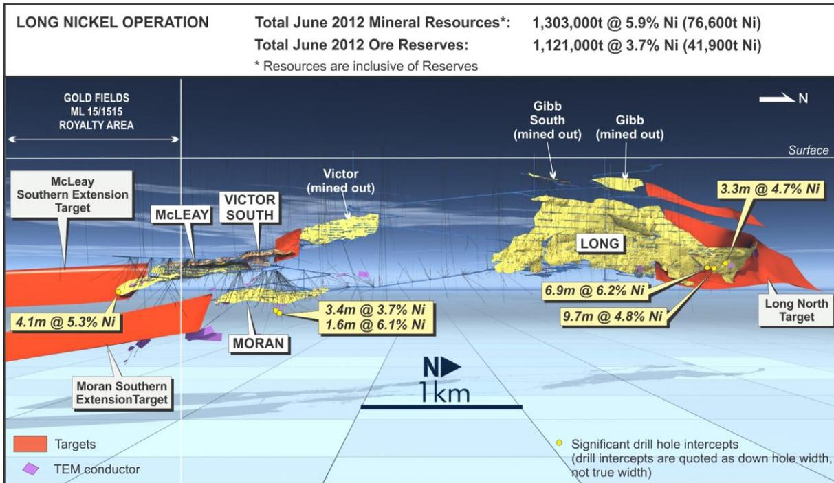
**Figure 4: Long Nickel Mine – Longitudinal Projection showing Target Areas, TEM Conductors and Significant Intercepts.**
