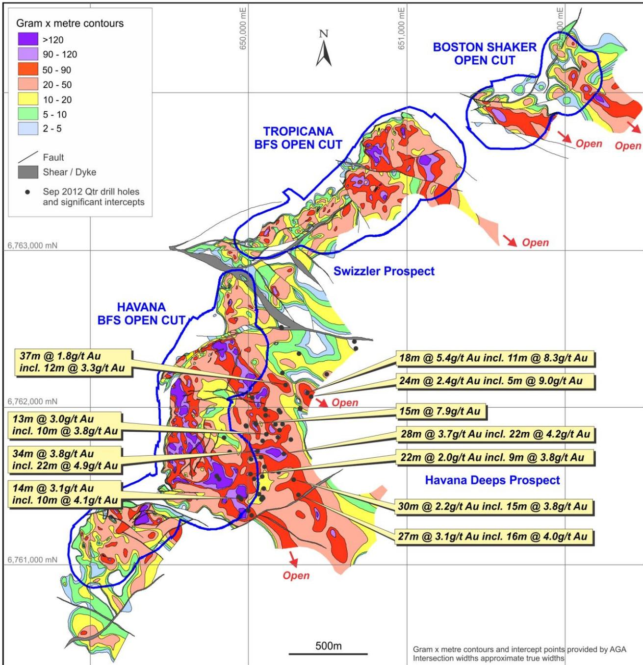
**Figure 3: : Tropicana JV – Proposed Boston Shaker, Tropicana, Havana and Havana South Open Pit Outlines, g/t Au x Thickness (m) Contours significant September 2012 quarter intercepts.**
