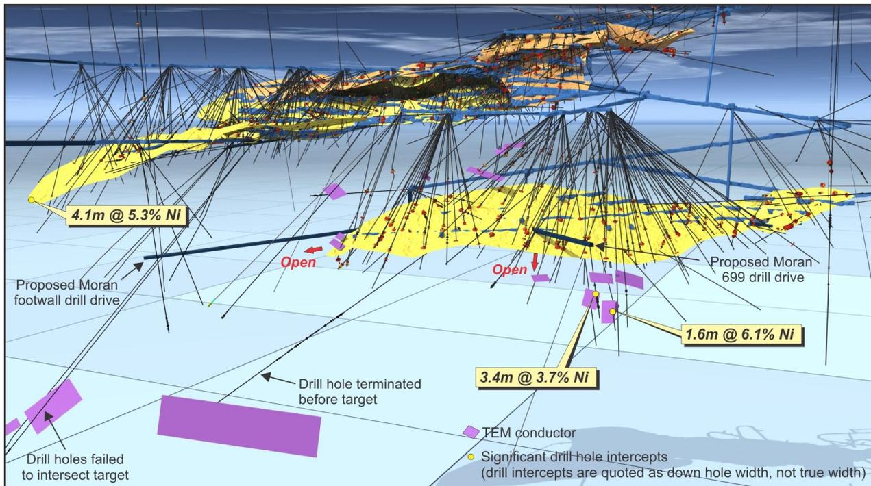
**Figure 5: Moran and McLeay 3D Isometric Model showing Nickel Shoots, Drillholes, Development and Intercepts outside June 2012 Mineral Resources.**
