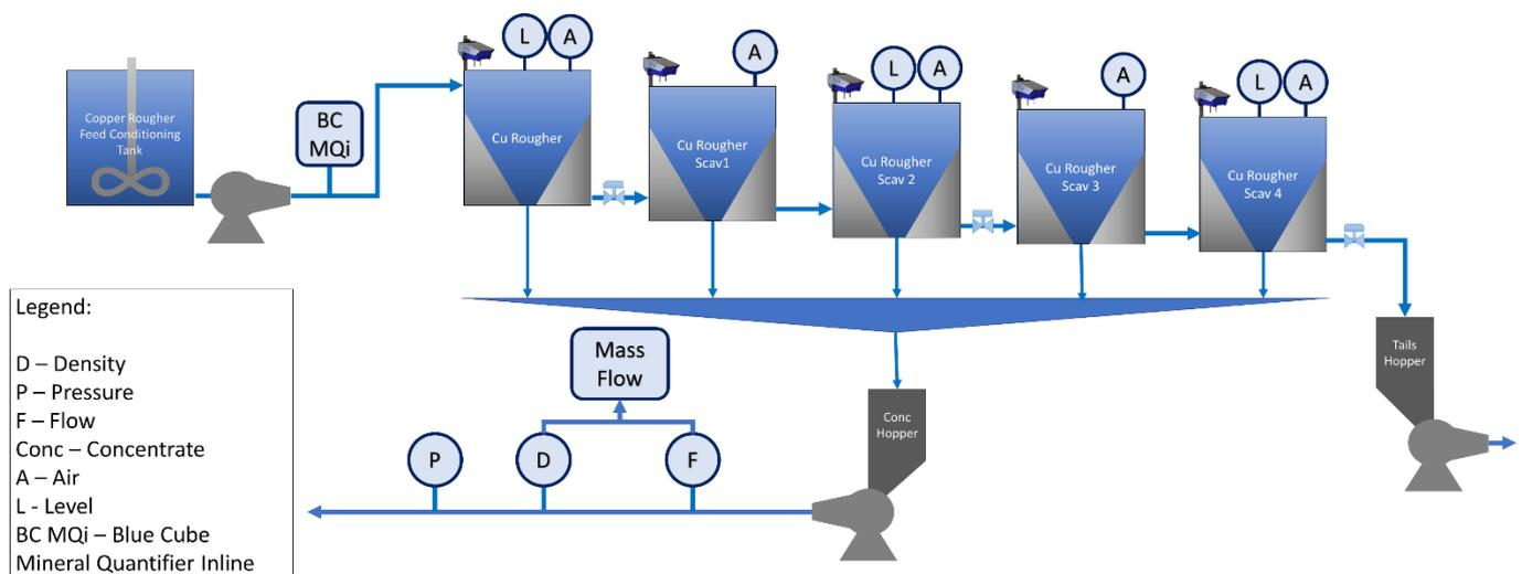
Figure 1 - Physical Layout of the Nova Copper Rougher-Scavenger Flotation Circuit at Nova.
