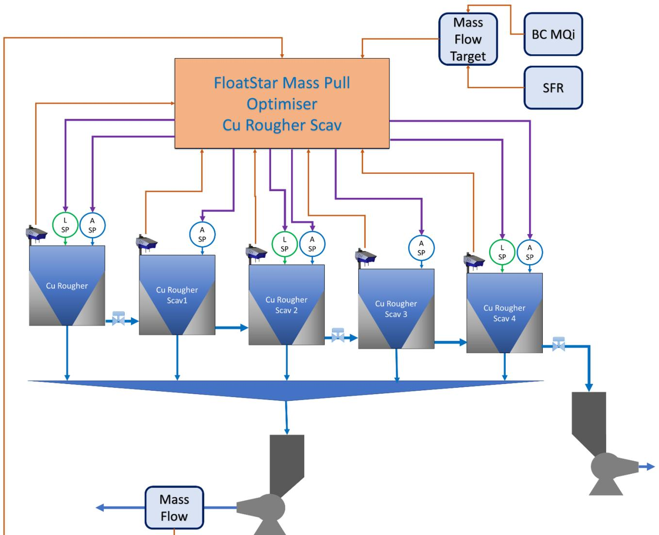
Figure 7 - StarCS Optimiser on the CRS circuit.
