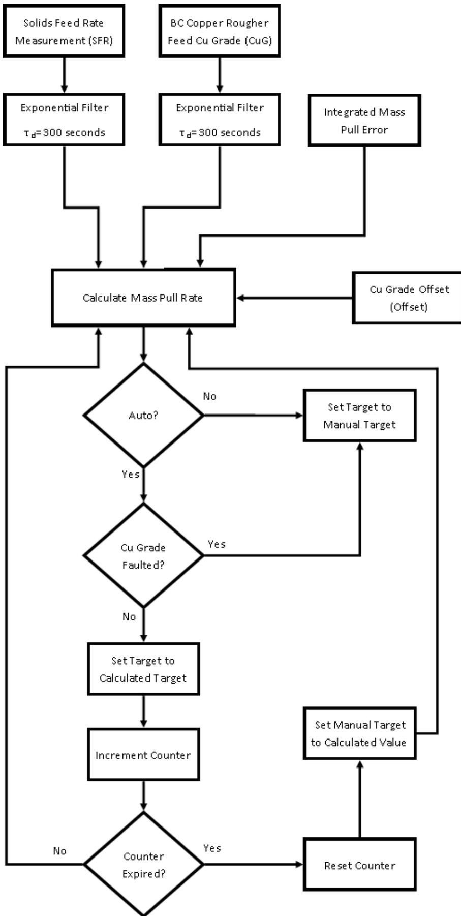
Figure 6 - Logic Diagram for calculation of Mass Pull Target.
