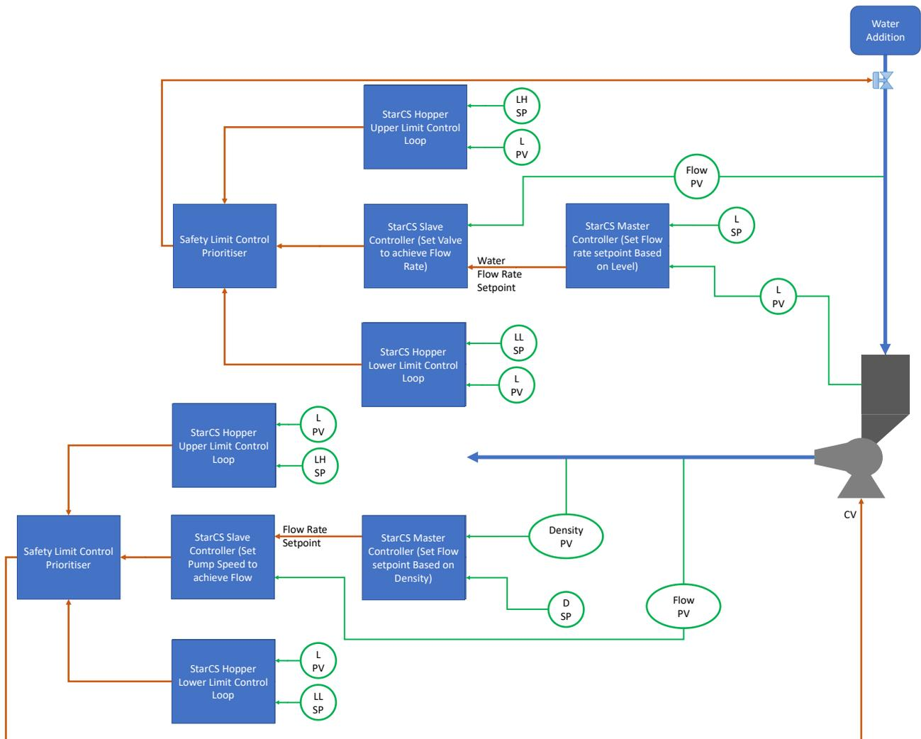
Figure 5 - Control strategy implemented on CRSC Hopper
