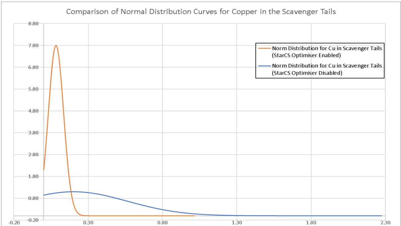
Figure 10 - Normal Distribution Curves for the copper in the Scavenger Tails with the StarCS Optimiser Enabled and Disabled
