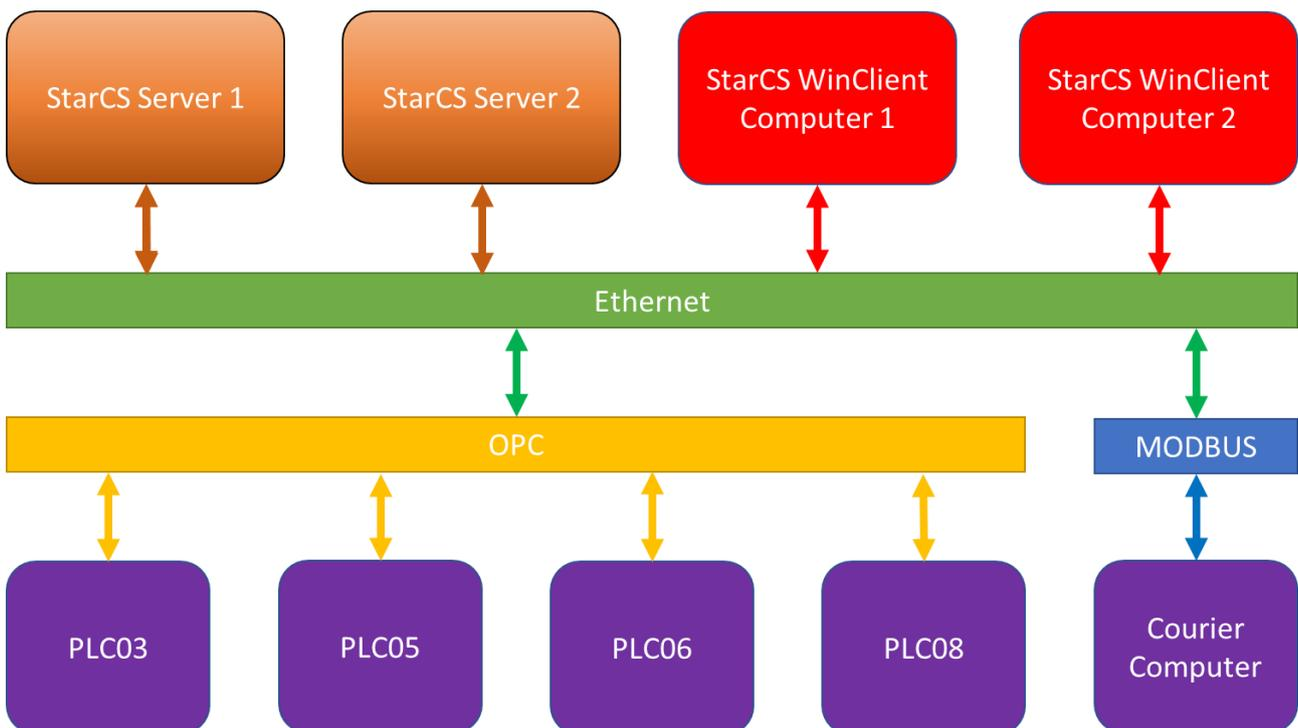
Figure 2 - Hierarchy of physical installation of StarCS at Nova.
