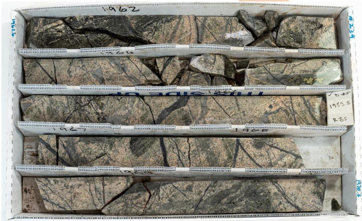
**Figure 2:** Drill core tray (HQ) from CPW0001DD showing high intensity of stockwork quartz-sulphide veining overprinting felsic gneiss and mafic schists. The upper section of HQ core in this photo is part of assayed interval 597.71 m – 599.54 m (1961' – 1967') which returned 7057 ppm Cu and 1295 ppm Mo for 1.62% CuEq<sup>3</sup>. The lower section of core is part of assayed interval 599.54 m – 601.37 m (1967' – 1973') which returned 2690 ppm Cu and 1509 ppm Mo for 1.33% CuEq<sup>3</sup>.
