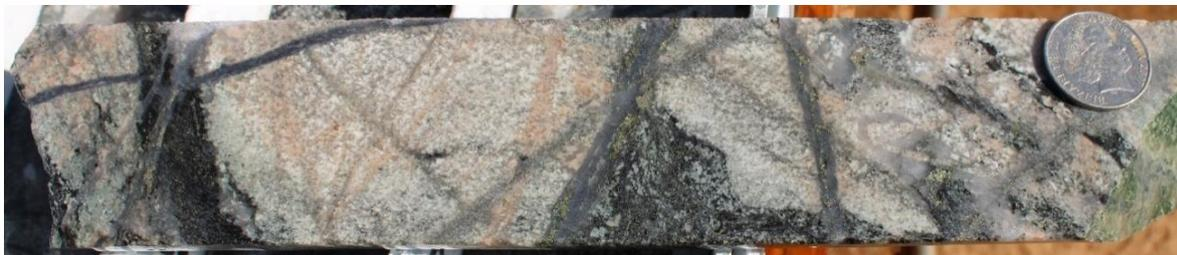
**Figure 1:** Porphyry-style alteration, veining and mineralisation in CPW0001DD at 594.66m. This section of HQ core is part of assayed interval 594.06 – 595.88 which returned 3936 ppm Cu and 745 ppm Mo for 0.92 % CuEq<sup>1</sup>.
