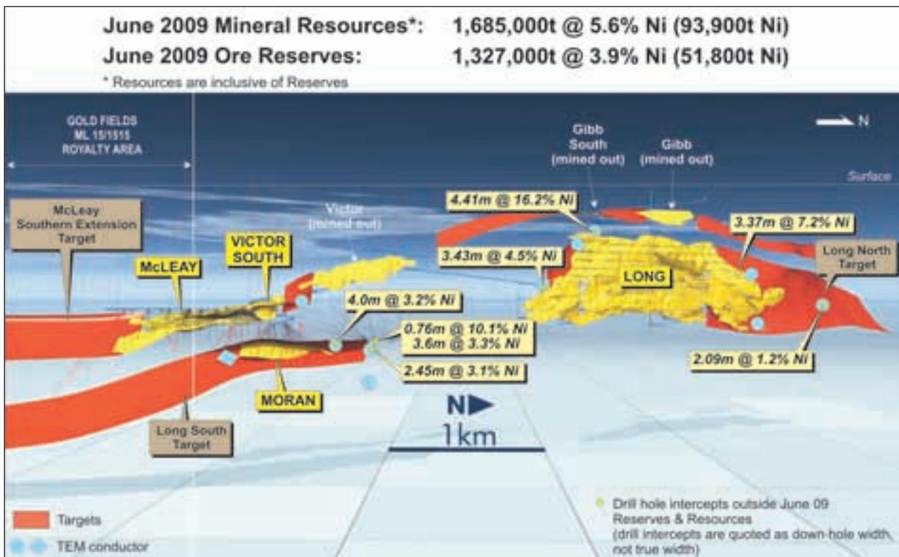
**Figure 2:** Long Nickel Mine - Longitudinal Projection Showing Target Areas, TEM Conductors, Significant Intercepts Outside Current Resources and Reserves and 2009/10 Exploration Targets
