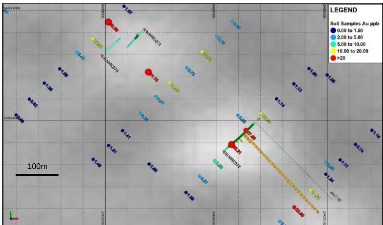
Figure 2 - Soil sampling and RC drilling traces at the Arcee Gold Prospect
