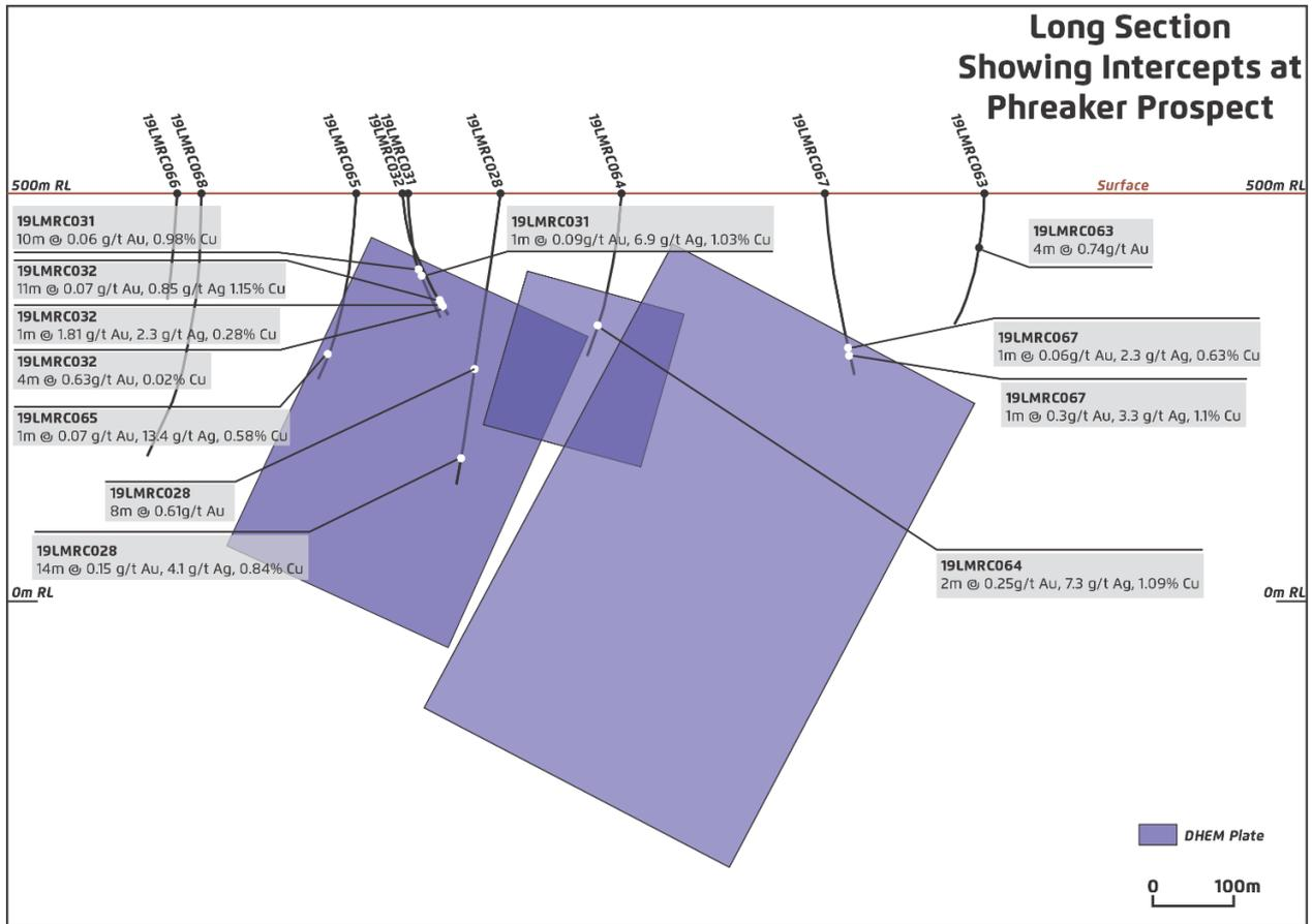
Figure 3 – Phreaker Long section illustrating RC drill intercepts and modelled DHEM plates
