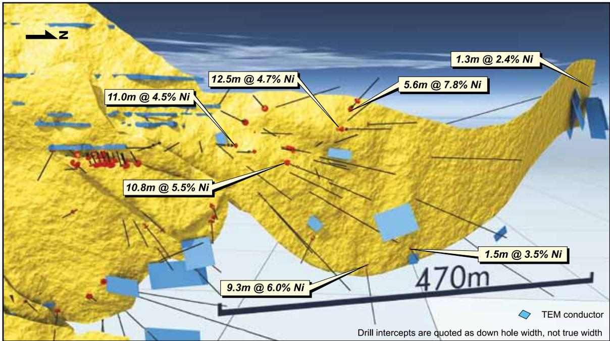
**Figure 4:** Long North - 3D Isometric Model Showing Nickel Shoots, Drill Holes, TEM Conductors, Proposed Development and Significant Intercepts
