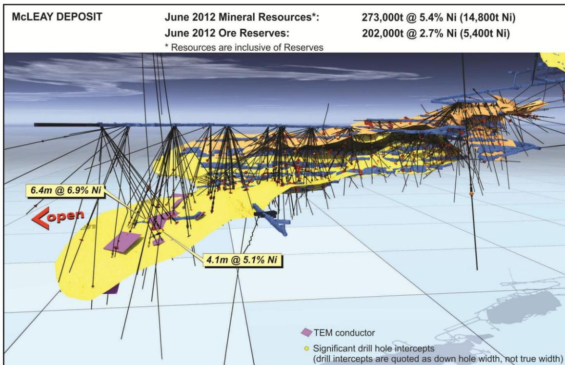
**Figure 5: McLeay – 3D Isometric Model Showing Nickel Shoots, Drill-Holes and Development.**
