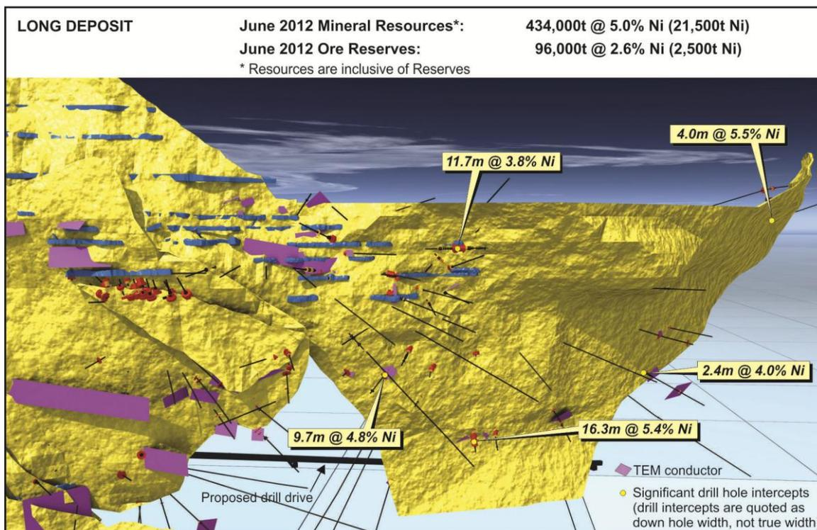
**Figure 6: Long North – 3D Isometric Model Showing Nickel Shoots, Drill-Holes, TEM Conductors, Proposed Development and Significant Intercepts.**
