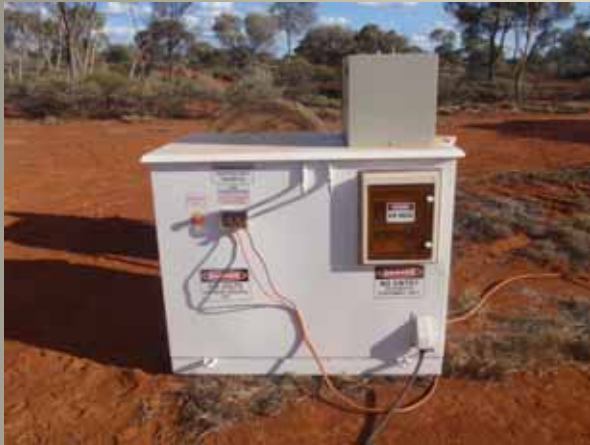
High powered TEM transmitter
