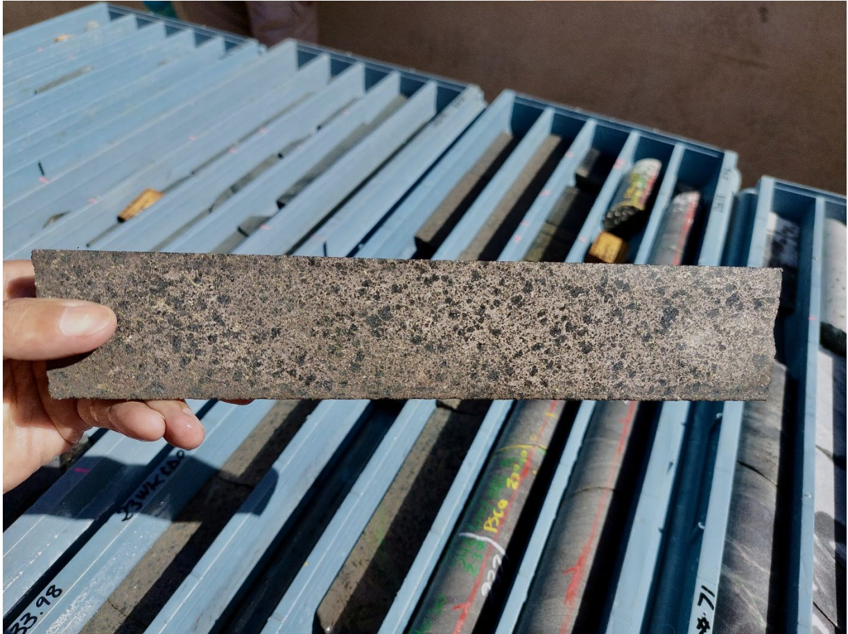
Figure 1: 23WKDD004 at approximately 234.0 m – Semi-massive “net textured” Ni-Cu sulphide mineralisation. The 2.89 m (True Width 2.63 m) interval assayed at 4.17% Ni, 0.83% Cu, 0.14% Co from 233.63 m (Table 1).
