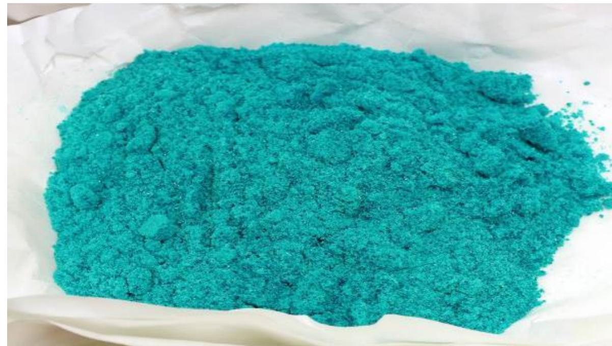
1) Photographs to the LHS are of the 1.6kg of nickel sulphate hexahydrate crystals produced in the metallurgical testwork. Photography by Karel Osten, Wood Plc
