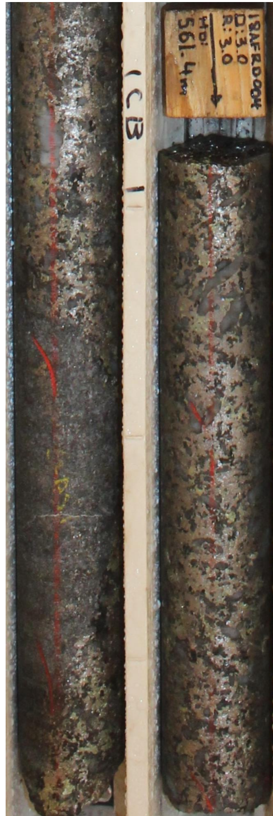
Notes: Pyrrhotite-dominated massive Fe-Cu-Zn sulphide mineralisation in a quartz breccia bounding a clast of finer grained and laminated rock characterised by higher sphalerite content. Core is NQ diameter (47.6mm).
