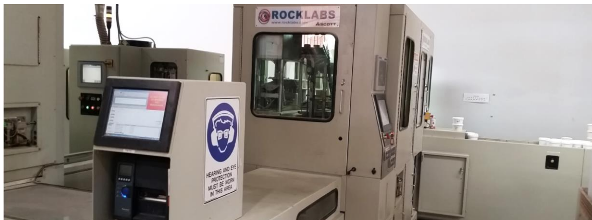
Automated sample preparation equipment at Tropicana Gold Mine laboratory
