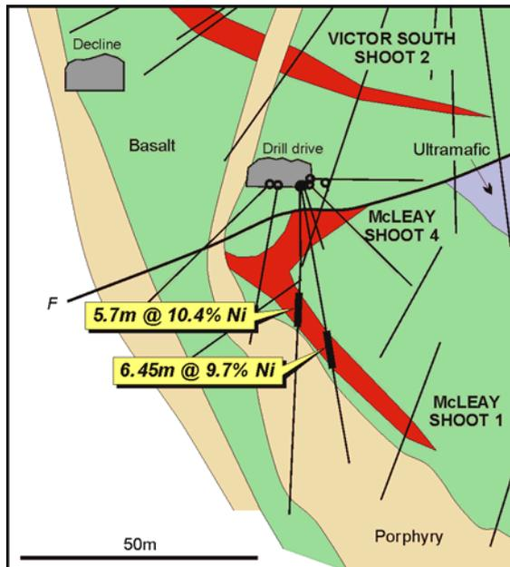
**Figure 1: McLeay Shoot 1 - 547,450mN Cross-Section Showing Resource Boundaries, Cross-Cutting Porphyry Dykes, Drill Holes and Significant Intercepts and the Location of the 460 Development Drill Drive**
