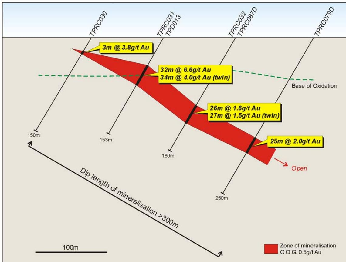
Figure 13: Tropicana JV – Tropicana Zone TPRC019-TPRC021D Cross-Section Showing Significant Drill Hole Results
