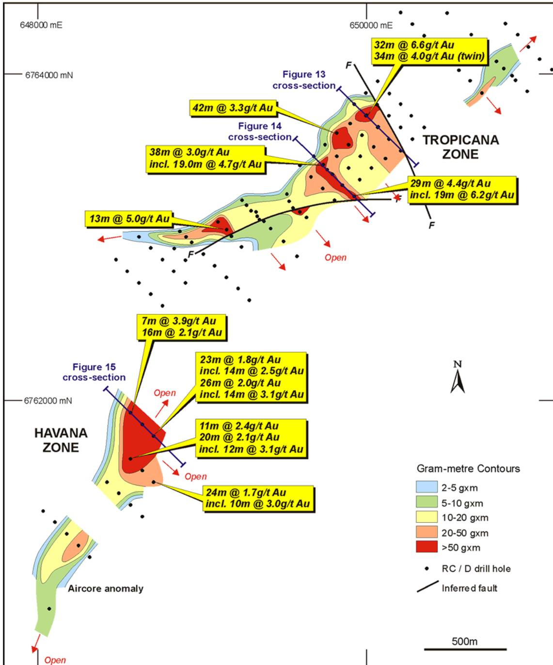
Figure 12: Tropicana JV – Tropicana Prospect Plan Showing Significant Intercept Locations, g/t Au, m Thickness Contours, and Location of Havana Zone
