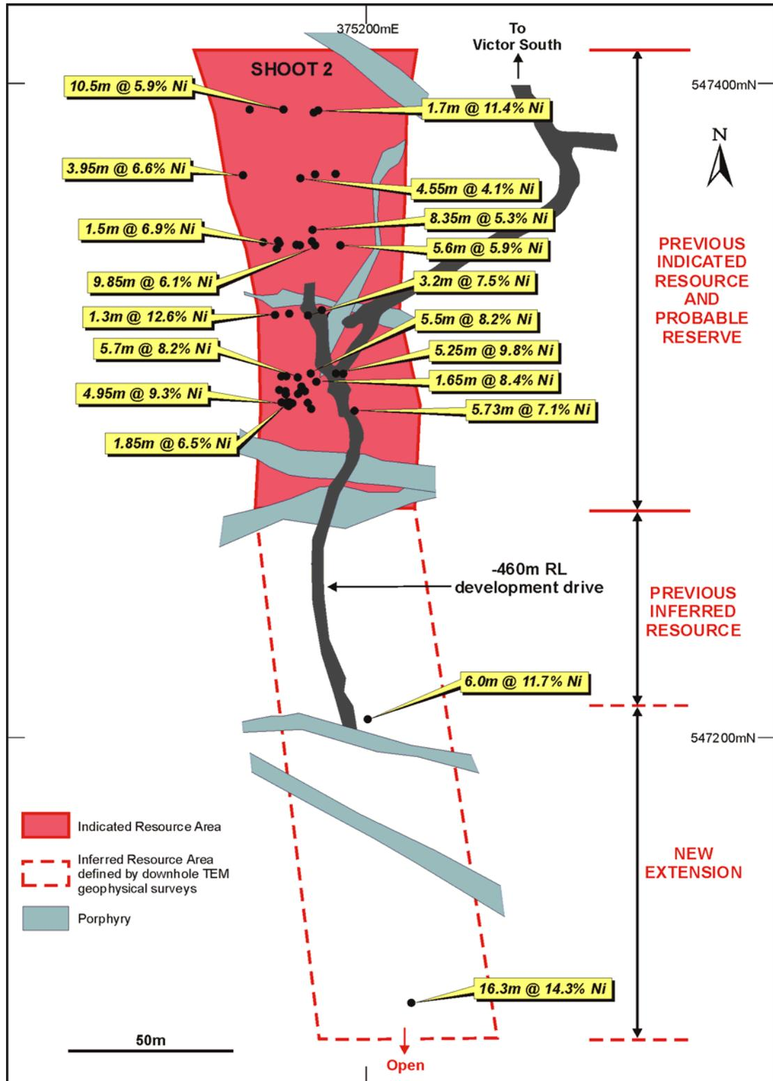
Figure 2: McLeay Shoot 2 Plan Showing Resource Boundaries, Cross-Cutting Porphyry Dykes, Significant Intercepts and the Location of the 460 Development Drive
