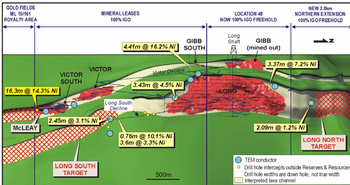
Figure 5: Long Mine Complex Longitudinal Projection Showing the Long South and Long North Target Access and Significant Intercepts Outside Current Reserves and Resources
