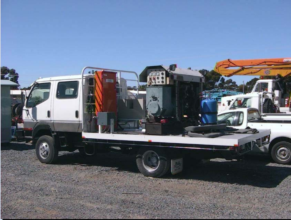
High power TEM transmitter truck developed in conjunction with Curtin University
