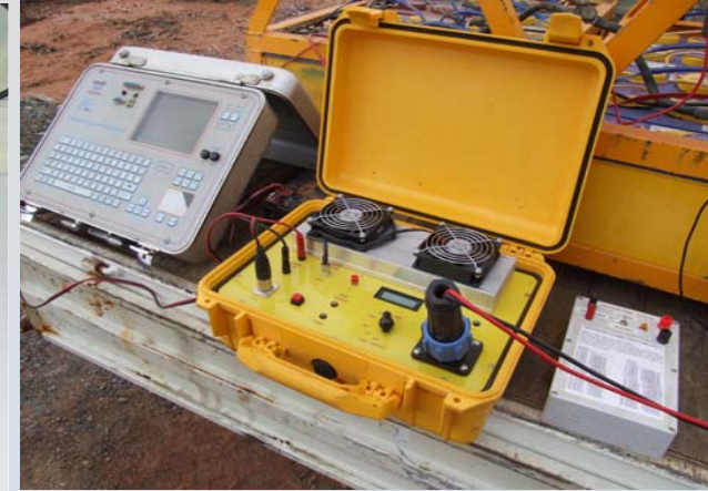
High powered TEM transmitter – 10 x more powerful than current systems in development by Independence / Curtin University
