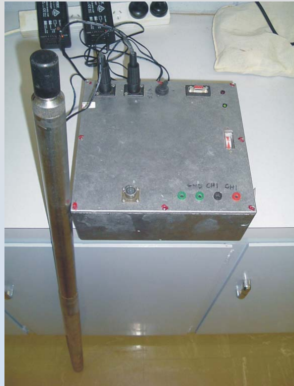
Down hole Mag TEM probe developed by Electromagnetic Imaging Technology
