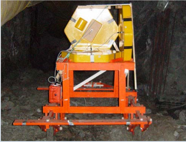
3 component underground TEM system developed by Independence / Curtin University
