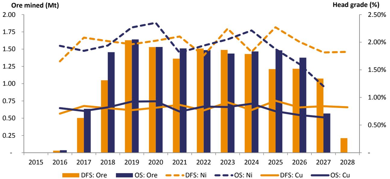
Figure 4: Production schedule for the Optimisation Study against the DFS showing mined ore (Mt) and grades (nickel % and copper %) for each financial year. The mining schedule has captured additional value through improving the available ore in FY17 and FY18. The schedule has also targeted higher grades earlier in the LOM (FY19 and FY20) with the deferral of the lower grades (FY26 and FY27).
