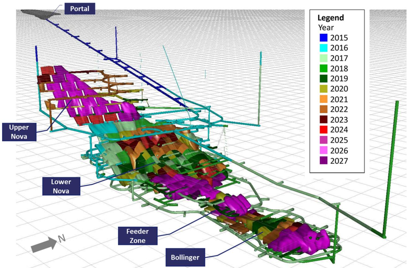
Figure 3: The development and stope sequence has been designed to improve the project NPV and accelerate early mill feed. A Centre-Out mining sequence focused on Lower Nova and Bollinger has maximised the number of stopes available along with targeting the highest NSR portions of the deposit.
