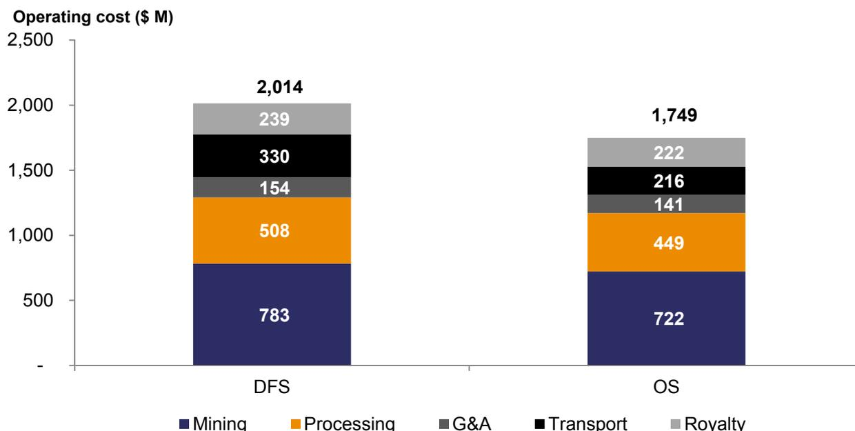
Figure 8: Graph showing the breakdown of LOM operating costs between the DFS and Optimisation Study
