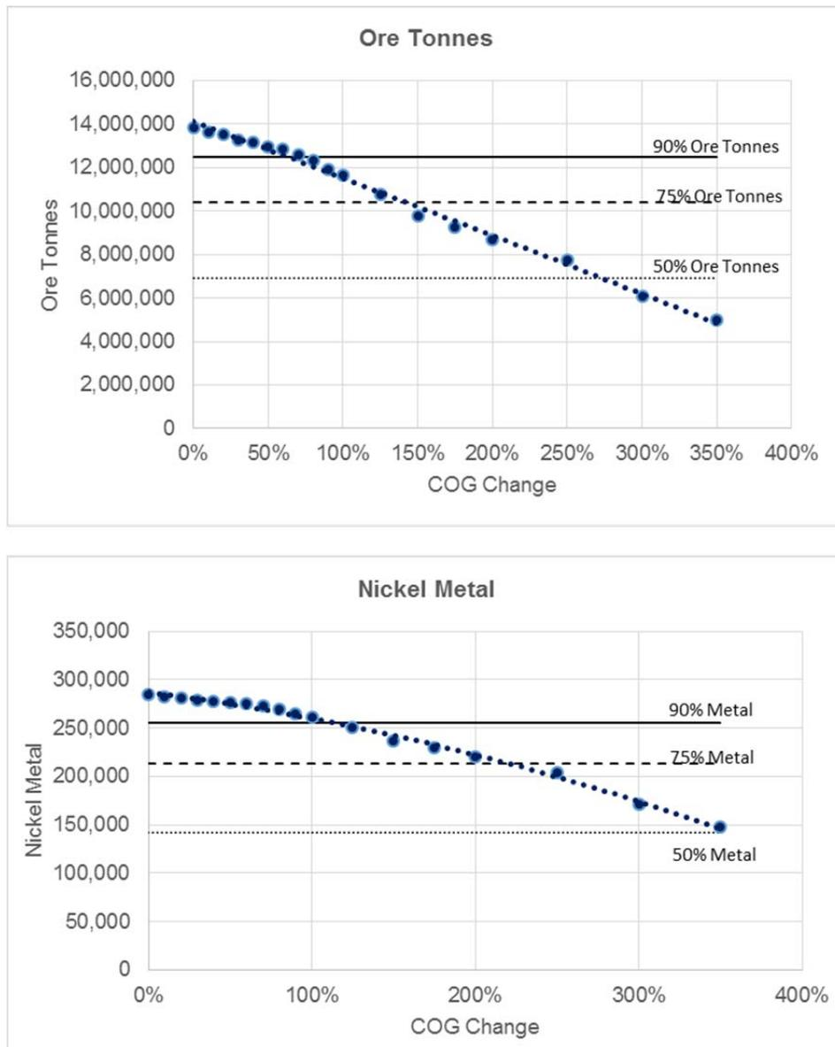
Figure 7: Graphs of a) Ore tonnes and b) Metal sensitivity for variable CoG's for the Optimisation Study physicals.
