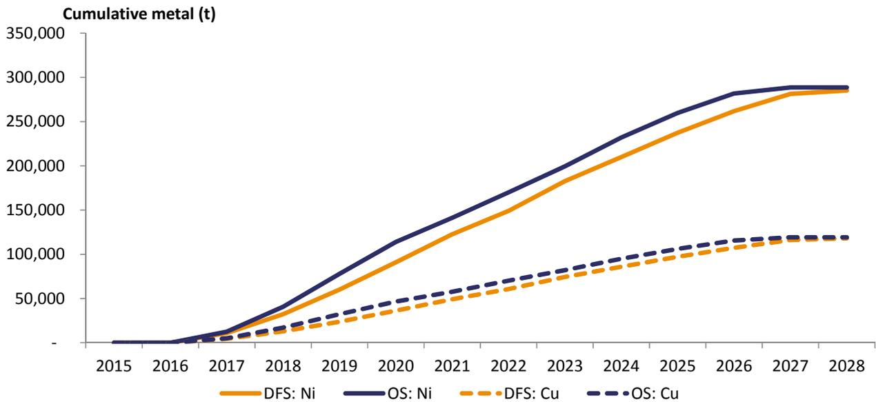
Figure 5: Graph showing cumulative metal as a comparison between the DFS and Optimisation Study (mined). The Optimisation Study has delivered an accelerated metal profile early in the LOM (on a like for like basis at 1.5Mtpa). Further improvements have been recognised to continue to improve the mining rates and throughputs.
