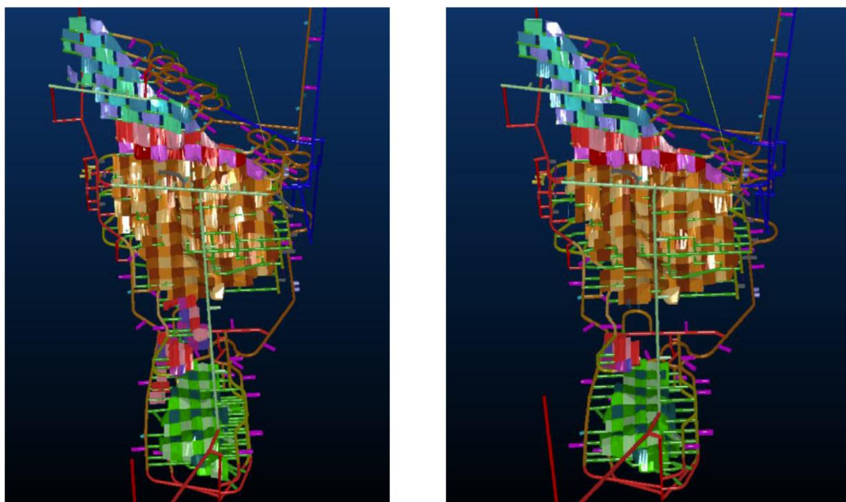
Figure 6: Image showing the a) stope & development design (on the left) with the Optimisation Study; and b) the stope & development design (on the right) with the low commodity price scenario. There is minor variance associated with the loss of lower value reserve tonnes on the margins of the Nova and Bollinger Deposits. The mine design would remain relatively unchanged.
