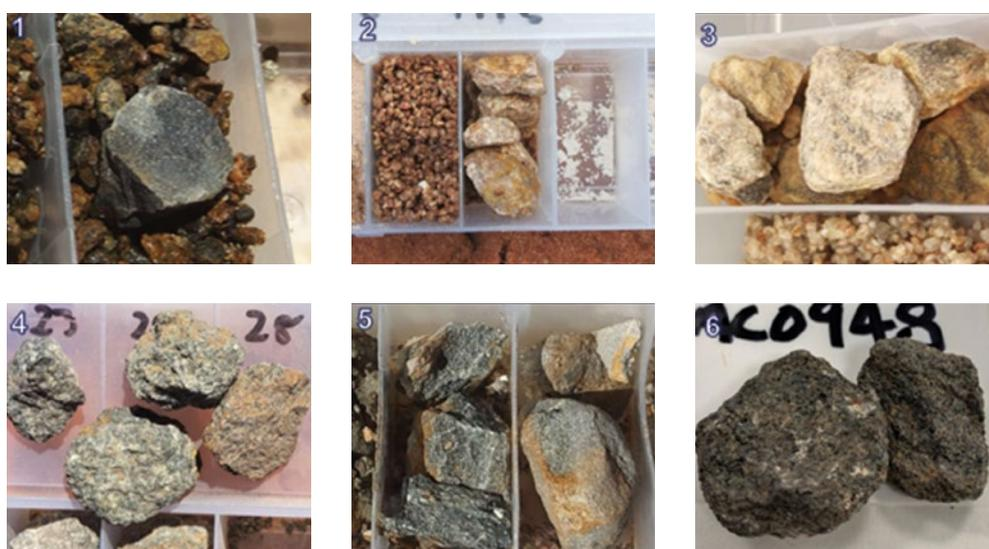
**Figure 31: Main lithologies in the 2021 and 2022 AC drilling**
