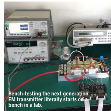
Bench-testing the next generation EM transmitter literally starts on a bench in a lab.
