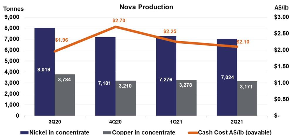
The Nova process plant milled 408kt of ore (1Q21: 394kt) at an average nickel and copper grade of 1.96% and 0.84% (1Q21: 2.12% and 0.89%), respectively for the Quarter. Tonnes milled were in line with the previous quarter and expected production rates, with one planned shutdown completed.
