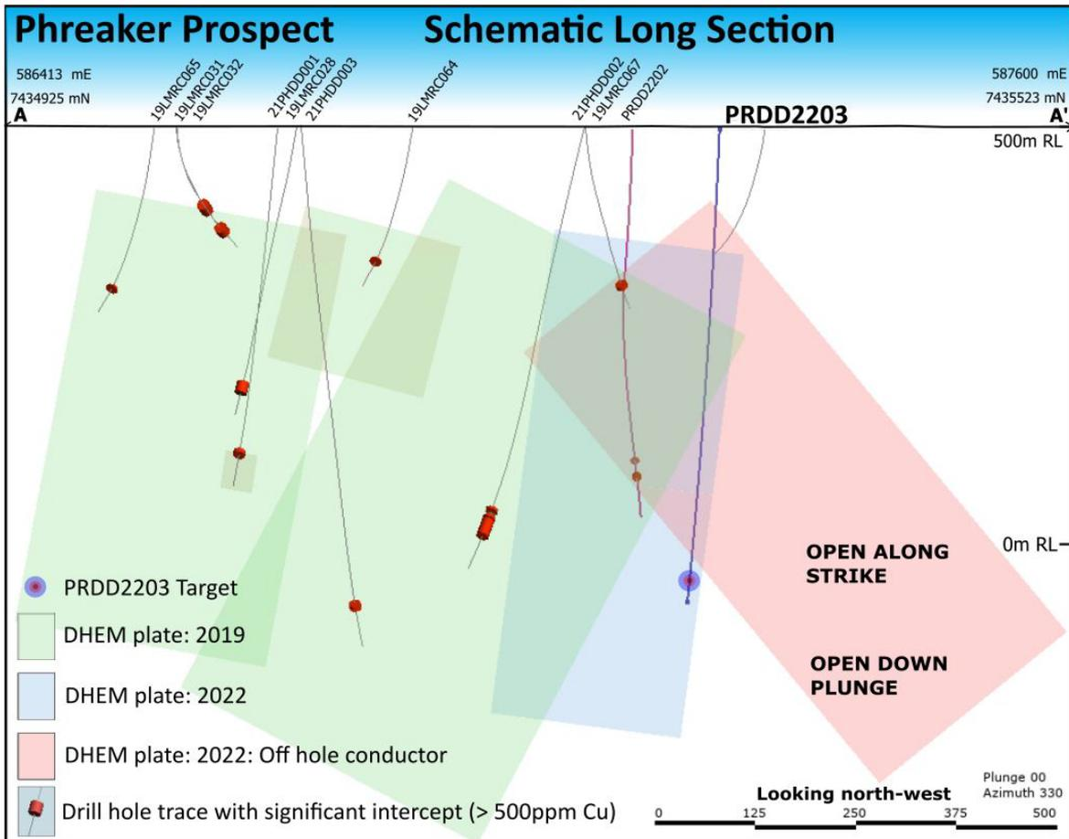
Figure 4 - Section of Phreaker showing the DHEM plates looking north-west
