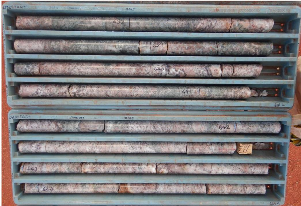
**Figure 3 – MAD213 from 637.60m to 644.90m showing a portion of the 120m+ intersect of coarse-grained pegmatite from the Manta seismic reflector**
