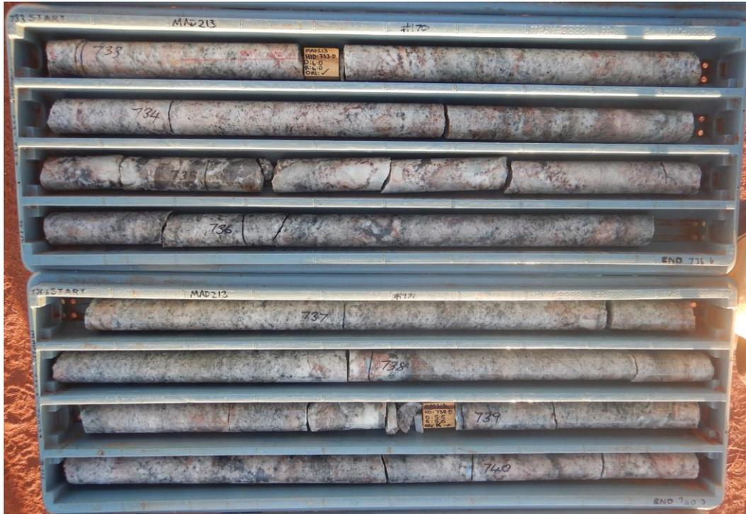
**Figure 7 – MAD213 from 733m to 740.3m showing a portion of the 120m+ intersect of coarse-grained pegmatite from the Manta seismic reflector**
