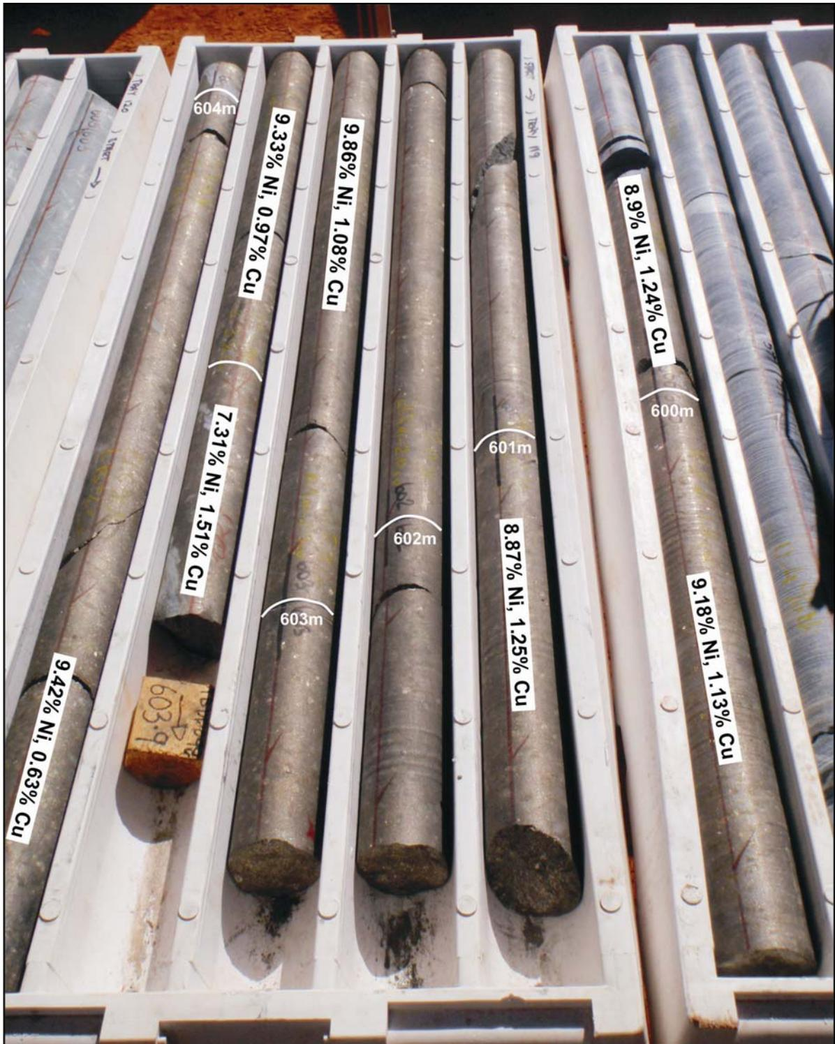
Figure 1: Duketon JV Rosie Prospect - TBDD098 Massive Sulphide Intercept 5.20m @ 9.13% Ni, 1.09% Cu, 0.21% Co and 7.09g/t PGEs (PGEs include 2.22g/t Pt, 1.74g/t Pd, 0.82g/t Rh, 1.79g/t Ru)
