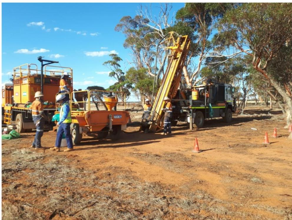
**Figure 1: Aircore drilling at Crossroads prospect with 'Zero Impact Rig', Burracoppin Gold Project**
