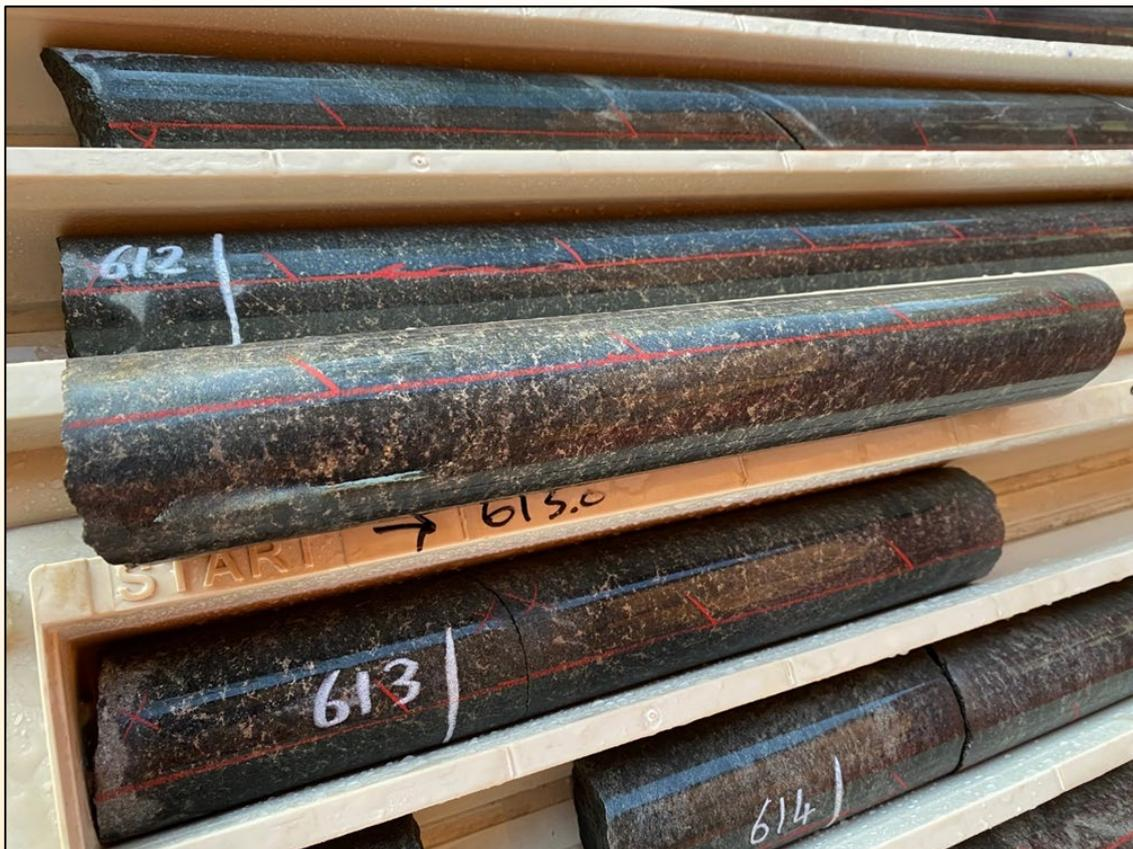
**Figure 1: Disseminated and moderately net-textured sulphides hole 20WKDD0002 611.75 – 613.57m**
