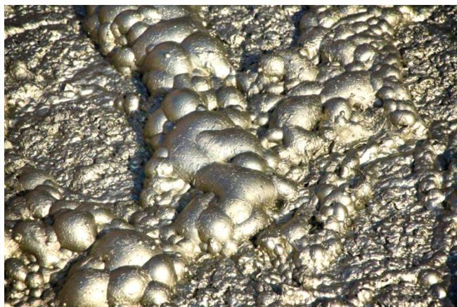
Copper flotation at Nova (14/10/16)
