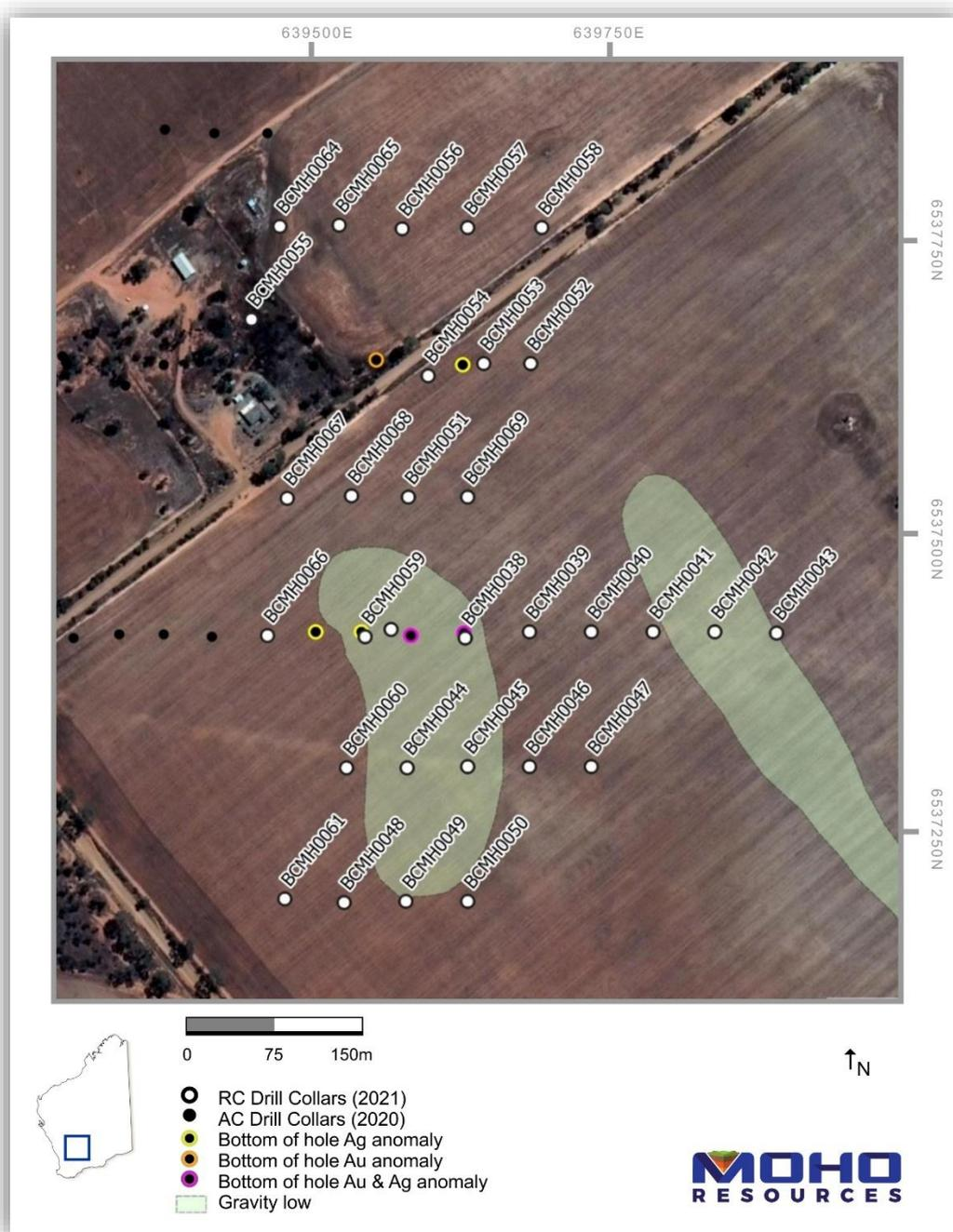
**Figure 2: Crossroads gold prospect drill hole location plan**
