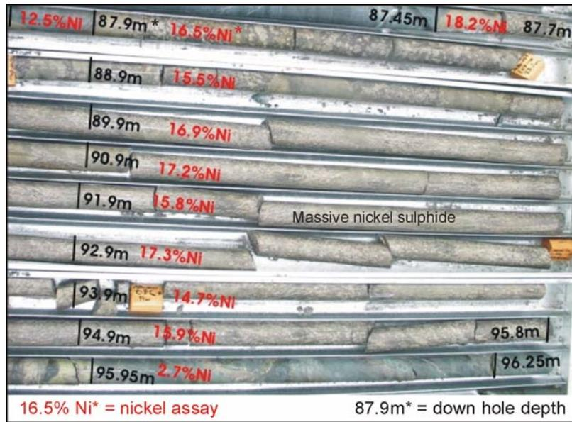
Figure 3: Hole MDU-041 Drill-Core Showing Down-hole Depth, Assay Boundaries and Nickel Grade
