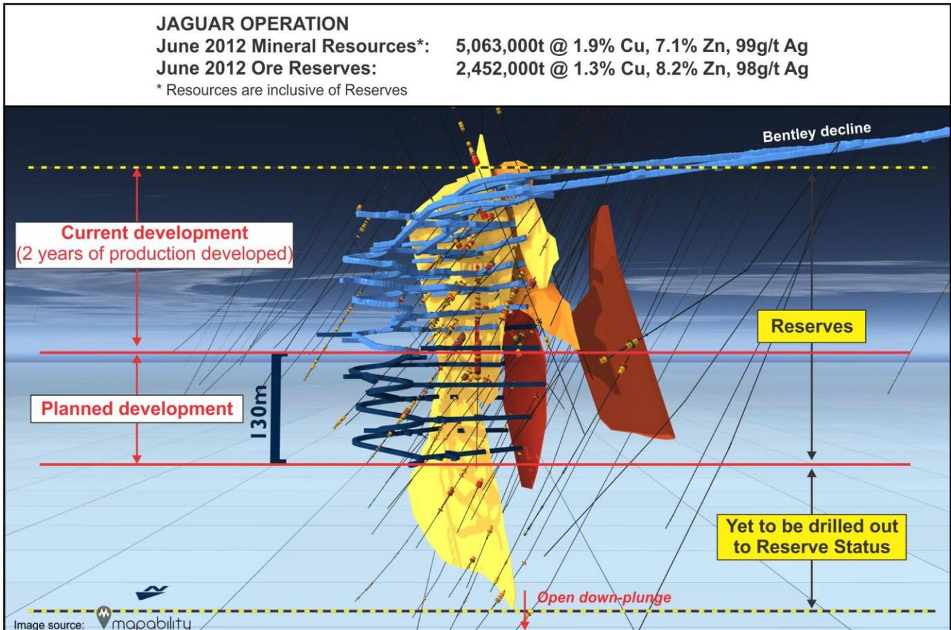
Figure 6: Bentley Longitudinal Projection, with completed and proposed development
