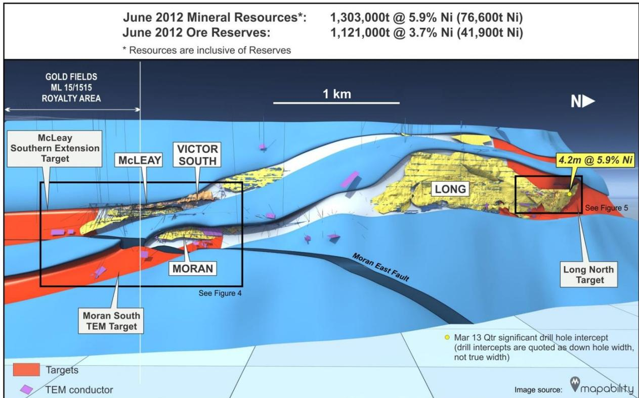
**Figure 3: Long Nickel Mine – Longitudinal Projection showing Target areas, TEM conductors and Significant March 2013 quarter Intercepts. Reference – IGO 19/10/12 Annual Report ASX Release for Resource and Reserve Estimates**
