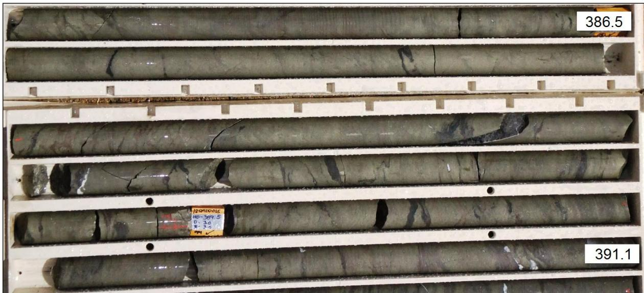
**Photo 5: Core photograph of higher grade Eureka massive sulphide intercept in 12SMDD015. Annotation refers to down hole depth.**
