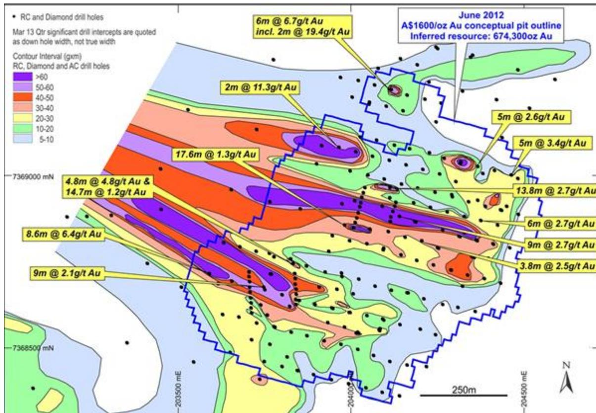
**Figure 9: Bibra Resource area – gram x metre Contours with A\$1,600/oz Au June 2012 Conceptual Optimised Pit Outline, RC and Diamond Drilling Collar Locations (AC Collars omitted) and significant March 2013 quarter drill results**
