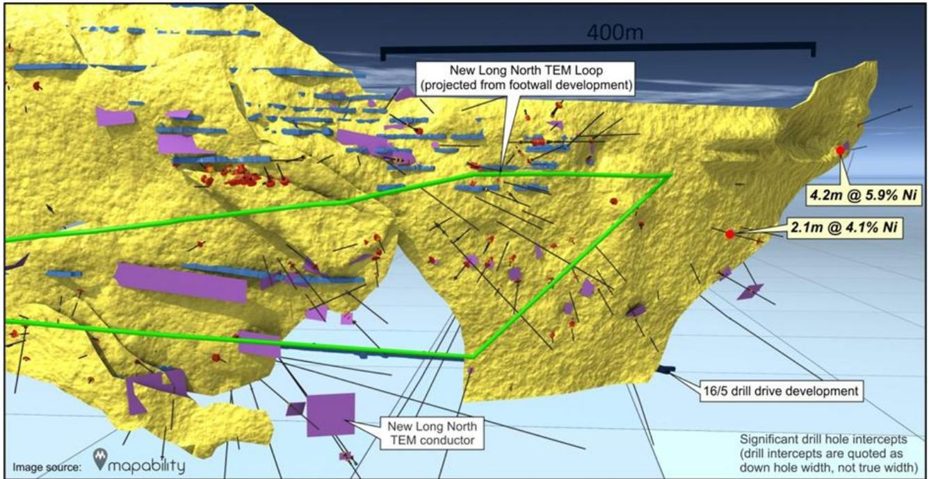
Figure 5: Long North 3D Isometric Model, Drill holes, TEM Conductors, Drill drive development, new TEM underground loop and Significant March quarter intercepts outside June 2012 Mineral Resources.
