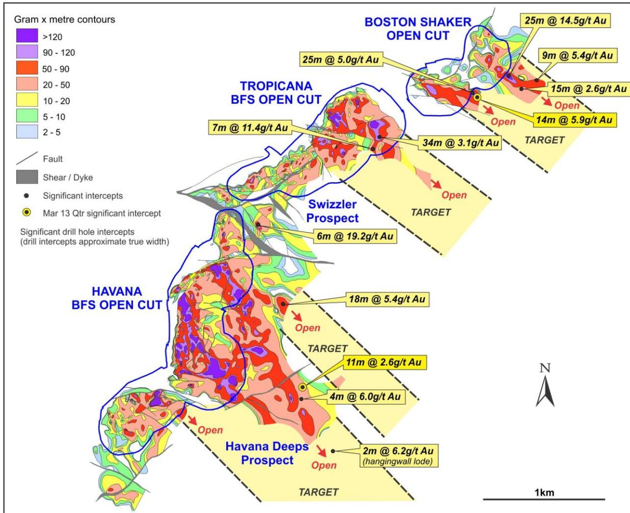
Figure 2: Tropicana JV – Proposed BFS Boston Shaker, Tropicana, Havana and Havana South Open Pit Outlines, g/t Au Thickness (m) Contours and significant March 2013 quarter intercepts
