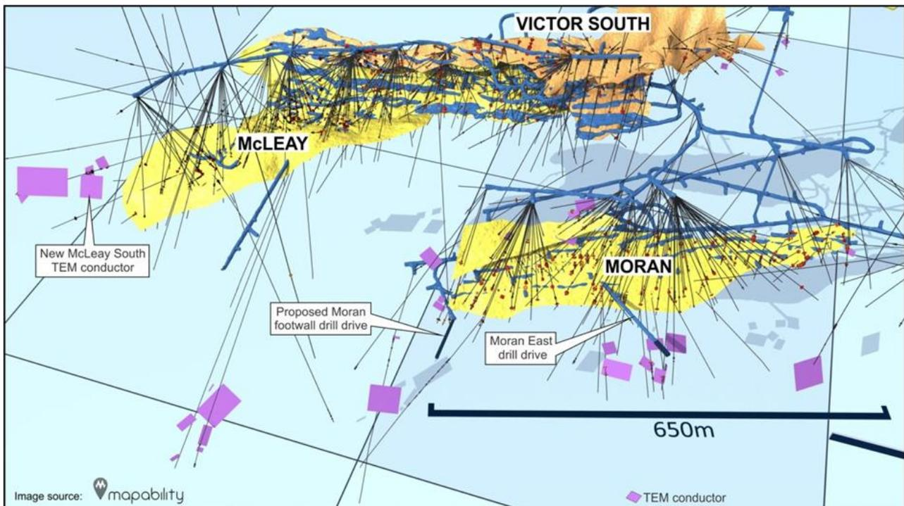
**Figure 4: Moran and McLeay 3D Isometric Model showing Nickel Shoots, TEM conductors, Drill holes, Drill drive and development**
