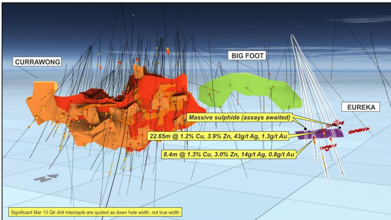
**Figure 8: Long Section looking to south east showing deposits, pierce points of current drilling, planned pierce points and modelled DHEM conductor.**
