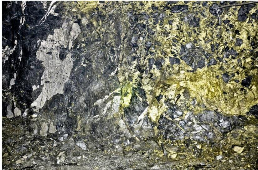
Photo 4: Bentley Footwall copper rich Azure zone: Development drive, showing semi-massive chalcopyrite mineralisation with brecciated texture.
