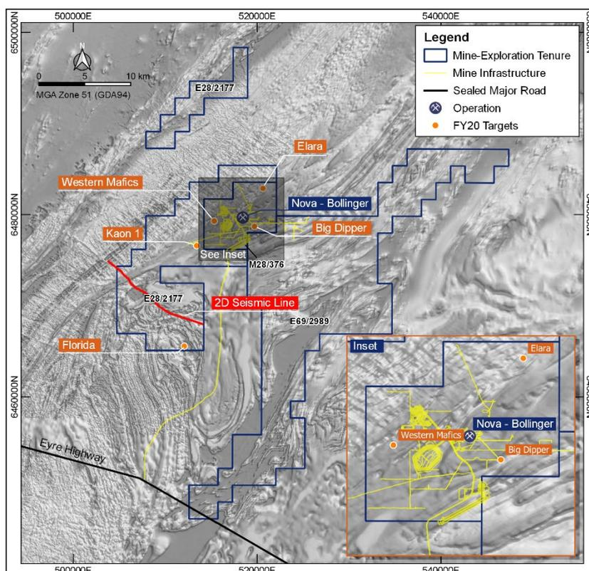
Aircore (AC) drilling on E28/2177 (west of Nova) was undertaken to map the bedrock geology and to follow-up geochemical anomalies identified from past AC drilling programs. In total, 284 holes were drilled with numerous M-UM intrusions with elevated nickel intersected for future follow-up. Results from AC and diamond drilling on E28/2177 continue to support the high prospectivity of the area southwest of Nova and follow up diamond drilling is planned for this area in 2020.
