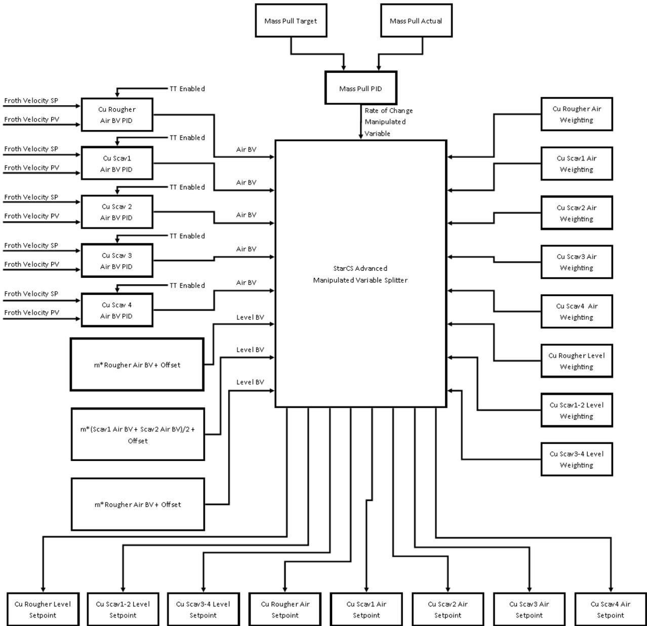
Figure 8 - Block diagram showing the main inputs and outputs required for the StarCS Optimiser.
