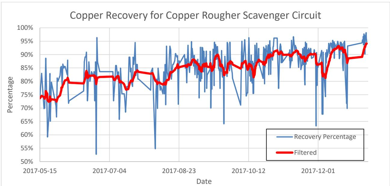
Figure 12 - Copper Rougher Scavenger Circuit Recovery
