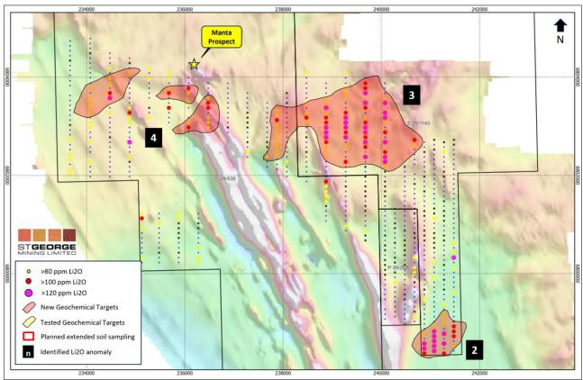
*Figure 4 – soil anomalies in the northern survey area.*
