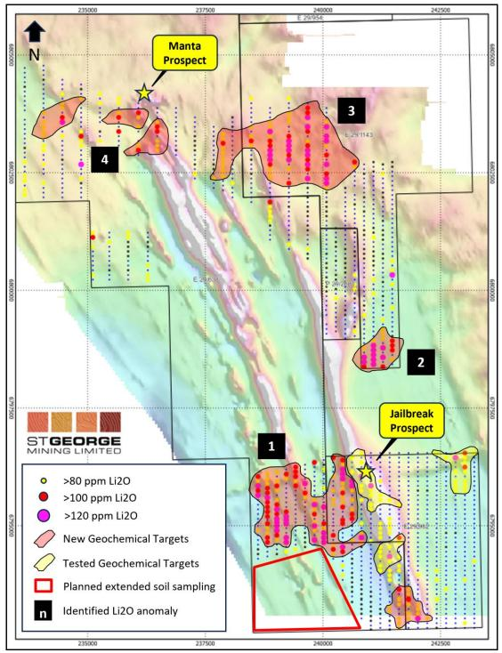
Figure 2 – map of Mt Alexander (overlying magnetic data) showing lithium in soil anomalies.
