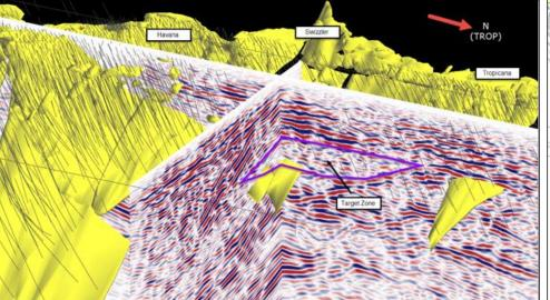
Seismic cube with a purple line indicating seismic target zone. 0.3 g/t Au wireframe in yellow and existing drill holes in grey.
