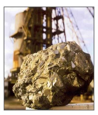
Nickel sulphides are very conductive and can be detected using electromagnetic geophysicial technology.
