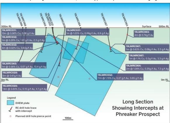
Phreaker Prospect long section - drill results, conductivity plates and planned diamond drilling targets
