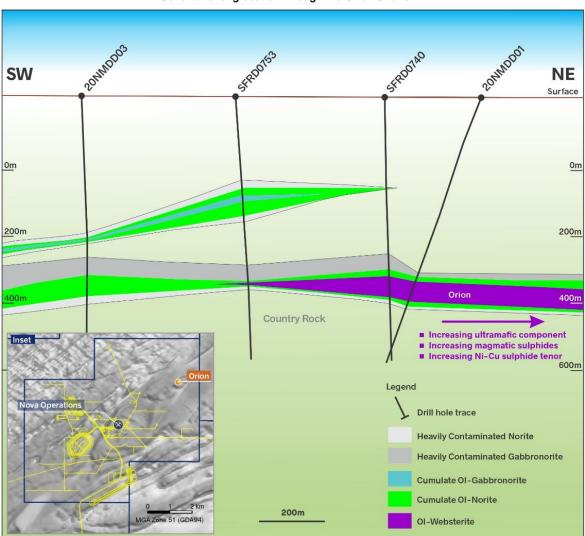
Schematic long section through the Orion Chonolith
